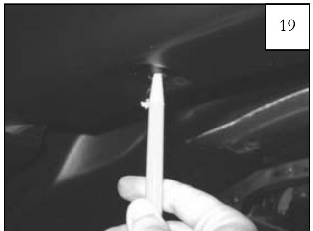
Hold the flare firmly on the fender. Using a grease pencil, mark four clip locations using existing holes in flare. See step 20.
