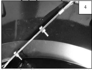
Insert the Screw/Washer assembly through the hole drilled in the end of the Front Main Flare and into the corresponding hole in the Front Bumper Piece. Two places. Install Clip CL1-0001 as close to outer edge as possible.
