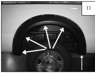
Ensuring proper flare placement, tighten all screws.
