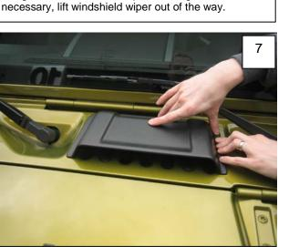
Press part into place. Apply 30 PSI to the taped areas for proper bond. The tape reaches maximum adhesive bond after 24 hours of contact. Do not wash vehicle for 24 hours.
