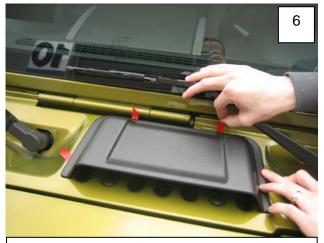
Maintaining part placement, begin pulling tape tabs while applying downward pressure to part.
