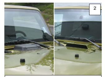
Without peeling liner from tape pads, position the part on the vehicle hood, centering over the air intake grill. You can position the hood scoop with the intake facing front or back as desired.
