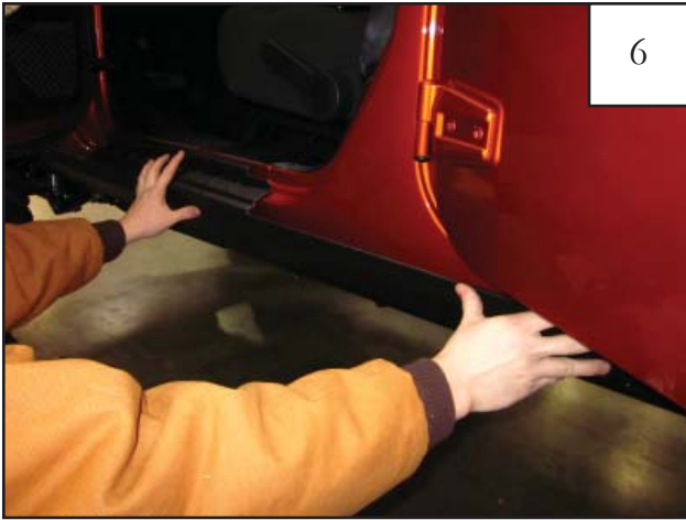
6 Place part on vehicle, making sure to line up edges of part with edges of vehicle and holes in part with clips installed in step 4. Ensure that all tape tabs are accessible.
