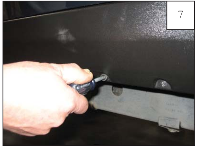
7 Using a #2 Phillips screwdriver, start a screw through each hole in side panel and through clips installed in step 4. DO NOT TIGHTEN SCREWS.
