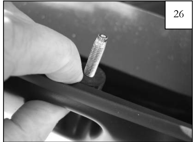
Place a 3/8" thick rubber spacer on each screw from the backside of the pocket. Threads must protrude through spacer for proper attachment of flare. All spacers must be installed prior to installation on fender.
