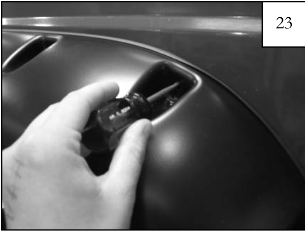
Hold the Front Flare in place on the fender, pressing firmly. Using the holes in the part as a guide, mark hole locations on fender (9 places).
