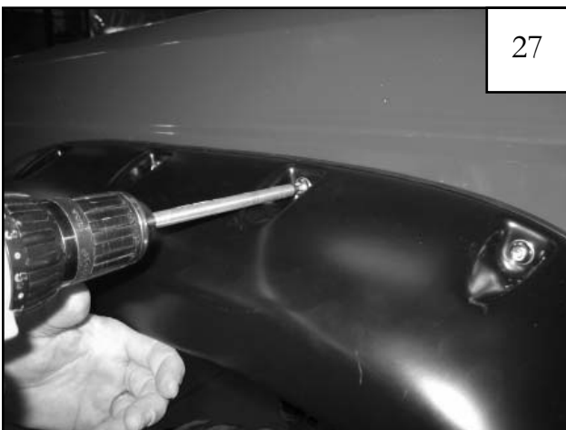
Start each screw with a T45 Torx bit in each pocket but do not tighten until all screws have been started. Note: Over-tightening screws may cause them to strip! Use a Torque setting of 24 inch/ounces.
