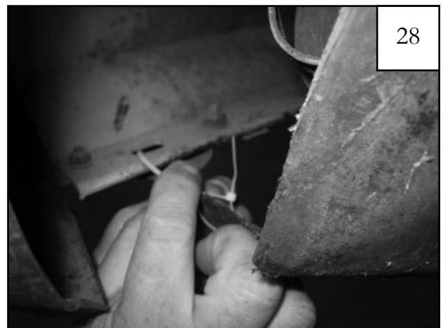
Optional: To secure splash shield, drill a hole and use a zip tie to attach it to the bumper.
